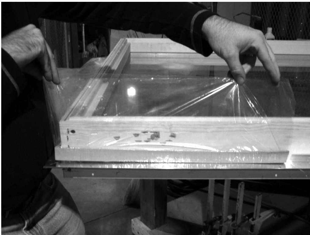
FIG. A1.8 Type B Material Applied with Polyethelene Liner
